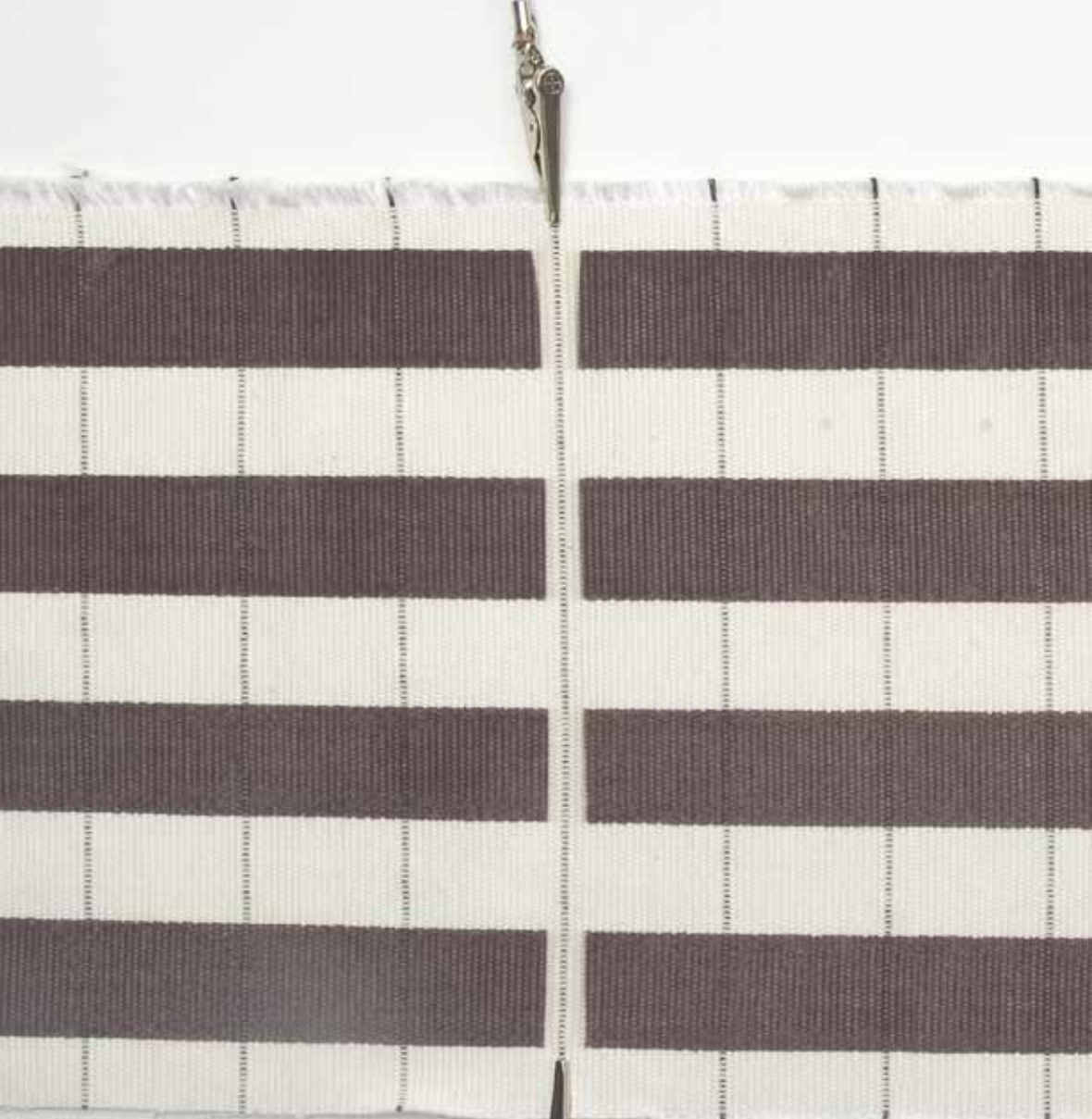
Dynamic textile pattern by Linda Worbin using thermochromic pigment and carbon fibers
