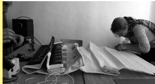
Constructing the inner fabric layer of the Energy Curtain
