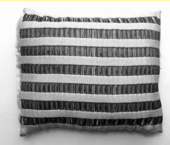
A second generation Interactive Pillow - a modern design, amplifying the electroluminescent fibre
